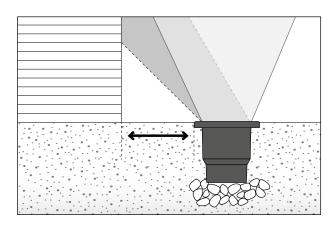
2. Provide a 30cm deep drainage with gravel. Position the luminaire loose into the gravel bed.
